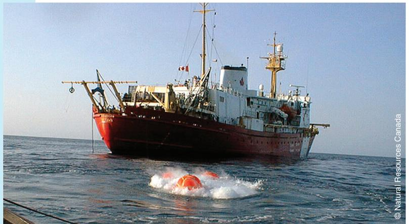
*Seismic airgun blasts cause bubbles to rise to the surface.*
