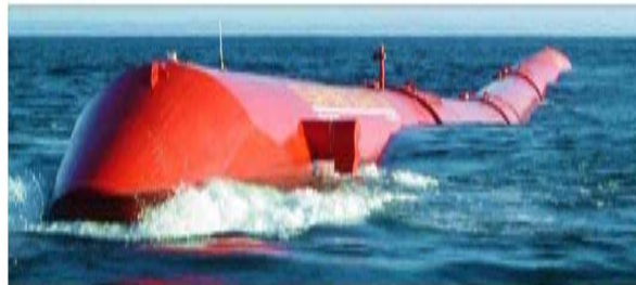
Attenuator Ocean Power Delivery Pelamis
