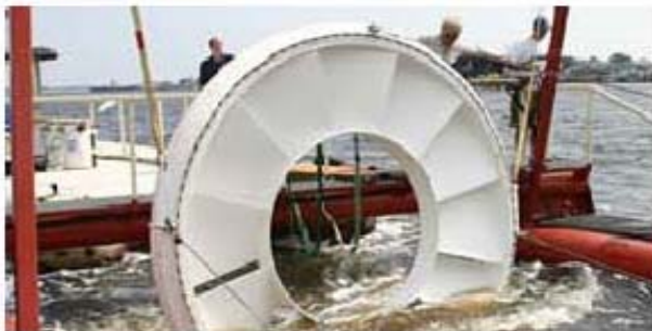
OpenHydro Open-Centre Turbine
