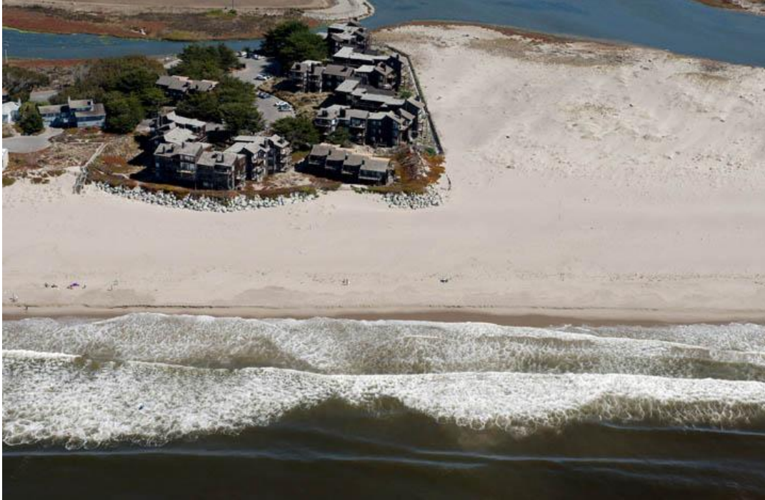
Figure 3-8. Aerial photograph of the southern end of the Pajaro Dunes-Sunset State Beach BECA, dated October 2013. The extensive development on active sand dunes is subject to wave attack and inundation from the adjacent mouth of the Pajaro River. Source: Adelman and Adelman
