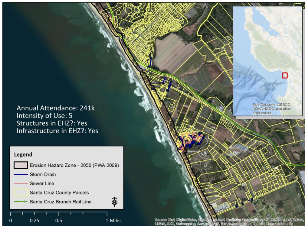
Figure 7-17. Erosion hazard zone - Manresa State Beach
