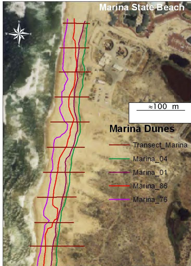
Figure16: Method of determining retreat rate at Marina Dunes study site. Long lines are dune-beach intersections of 2004, 2001, 1986 and 1976 plotted on the 2001 digital aerial photograph. The short lines are ten transects across the images used to determine average retreat rates at the site. Each of the four study sites (Marina, Stillwell, Resort, Condominiums) were similarly assessed.
