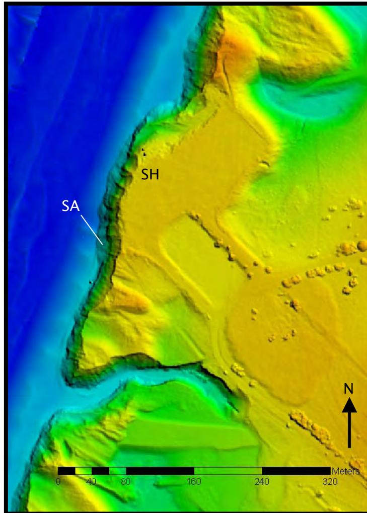
Figure 18: Shaded relief image from 2004 LIDAR data shows former Stillwell Hall site (SH). Sand aprons are visible at the base of steep sea cliffs (e.g., SA). Canyon (near the scale bar) rapidly eroded in response to broken storm drain. The storm drain had been undercut by coastal retreat. See Figures B8 and B9 for oblique ground photographs of the mouth and apex of the canyon. Data courtesy of Dave Lott (Monterey NOAA).
