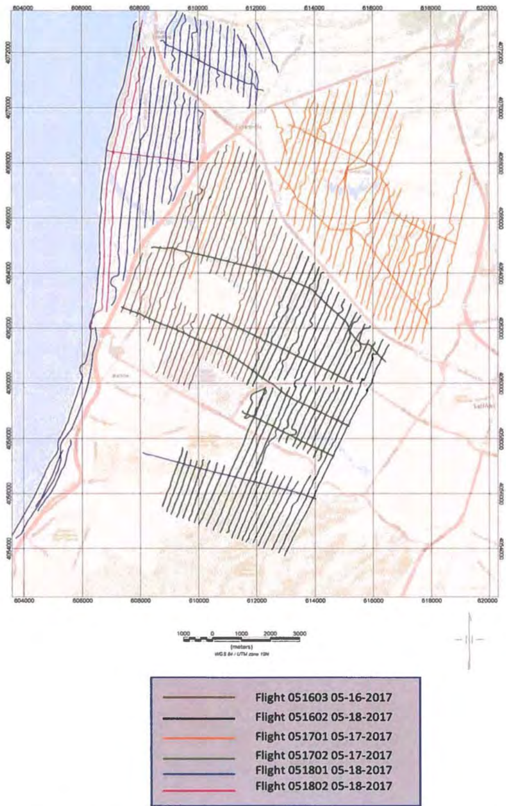
Figure 3: As-flown flight lines in the MCWD SkyTEM data acquisition. From the AGF "QA/QC and Preliminary Laterally Constrained Inversions Report from the Airborne Electromagnetic Survey of Selected Areas Within the Marina Coast Water District"
