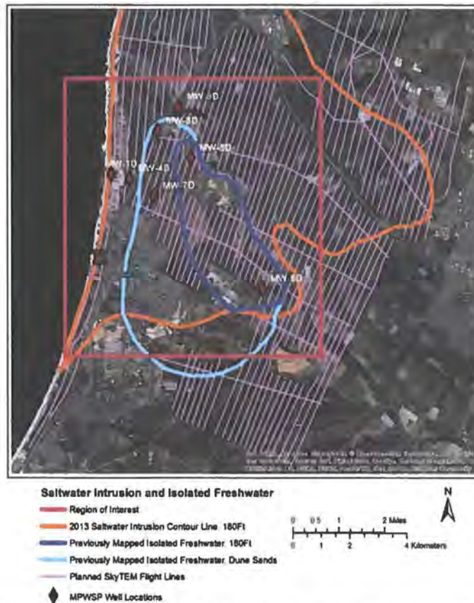
Figure 1: Region of interest (pink box) showing previously mapped saltwater intrusion (orange) extent in the 180-Ft Aquifer and the previously mapped extent of the isolated freshwater (light and dark blue) in the Dune Sand and 180-Ft Aquifers. Also shown are the 7 MPWSP well clusters with geophysical borehole logs as well as continuous data loggers in all screened intervals, and the planned SkyTEM flight lines for the AEM data acquisition
