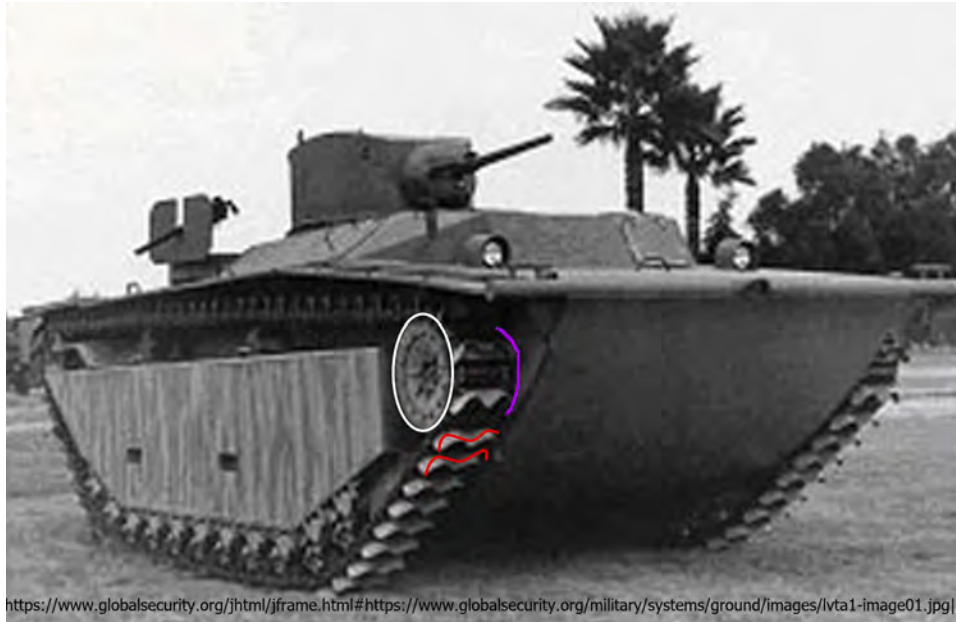
Figure 3. This LVT-A is an amphibious tracked vehicle similar to those at the Mating Amtracks site. Note the distinctive “M-shaped” treads (red.) A drive wheel (white) is mounted on a drive shaft that passes through a large hole in the hull (purple) near the bow-end.
