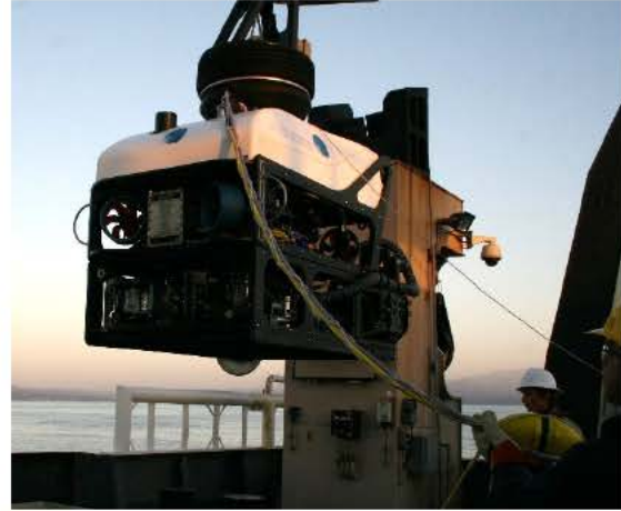
Figure 2. The GFOE ROV, Yogi , being deployed off the NOAA vessel Reuben Lasker .
