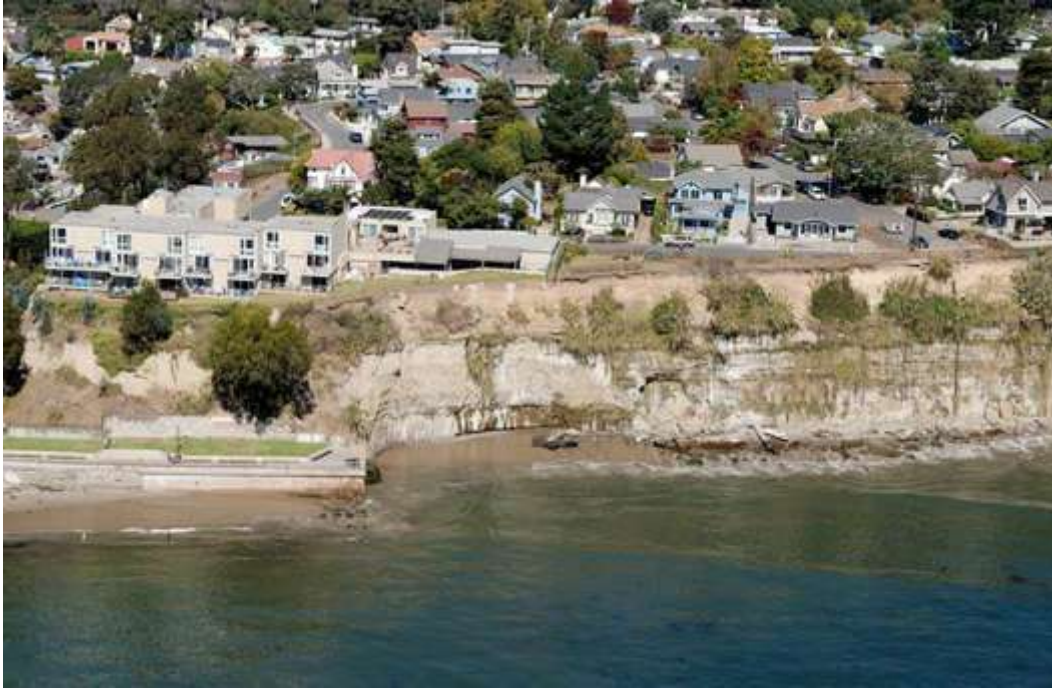
Figure 3-7. Aerial photograph of the western end of the Depot Hill BECA, dated October 2013. Note the significant sea cliff erosion, which threatens public and private infrastructure. Source: Adelman and Adelman
