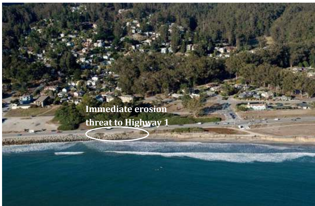
Figure 3-4. Aerial photograph of the northern section of the El Granada County Beach BECA, dated September 2013. Bluff erosion is currently threatening to undermine Highway 1. Source: Adelman and Adelman
